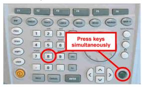
2. Switch the instrument on and keep PRESET and 8 pressed for at least 5 seconds after the startup screen has appeared on the screen.
