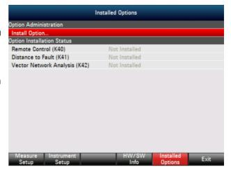
If the correct key code is entered, the R&S FSH displays "Installation successful", and the option is marked as "Installed" in the option list (example: Remote Control (K40)).
